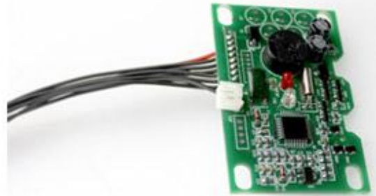
Pcb board:no Independent clock chip MF chip often loss information
